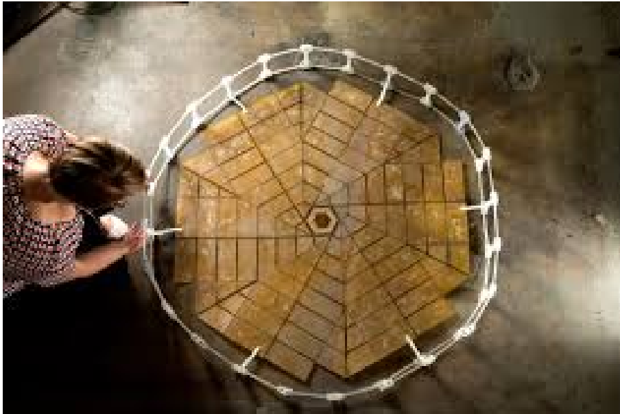
Figure 1.2: Origami based deployable solar panel for space application, Image credit: NASA
