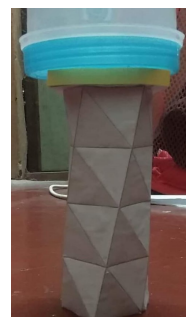
Figure 2.10: Hard-Deploy-Hard-Collapse Model under loading
